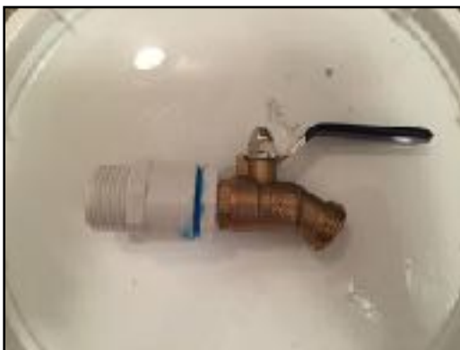
Figure 11 Allow PVC to dry
